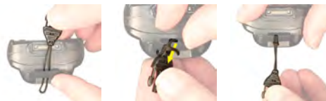
1. Thread small cord loop through connection point. 2. Thread connector through opening of loop. 3. Pull connector to tighten knot.
